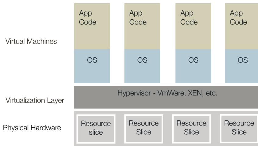
Figure 1. Architecture of traditional virtualization with Virtual Machines
